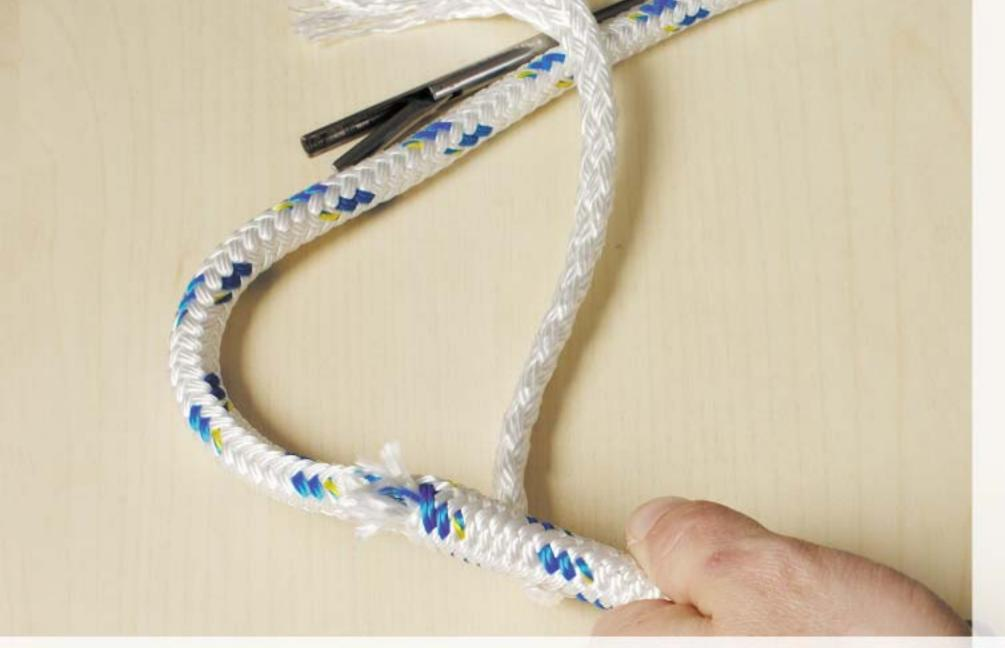
"Milk" the cover down over the core so that the cover on the inside and the other core finish flush with each other.
