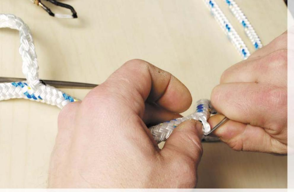
Pull the core out of the cover at the two 30 cm markings.
