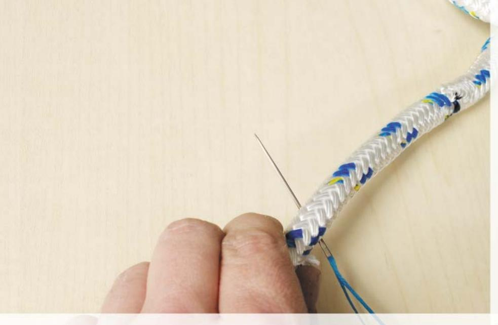
Sew through the splice on sides of the centre several times to prevent any movement of the core.
