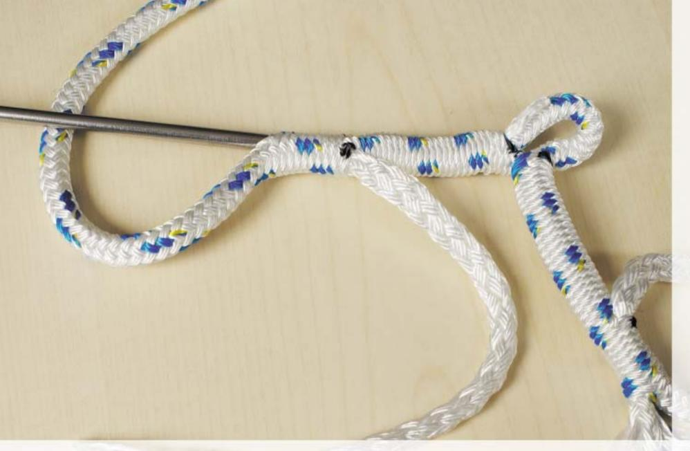
Now insert the other core at the other 15 cm mark and push it through to the 30 cm mark where the core came out. If possible exit 20 cm past the 30 cm mark.
