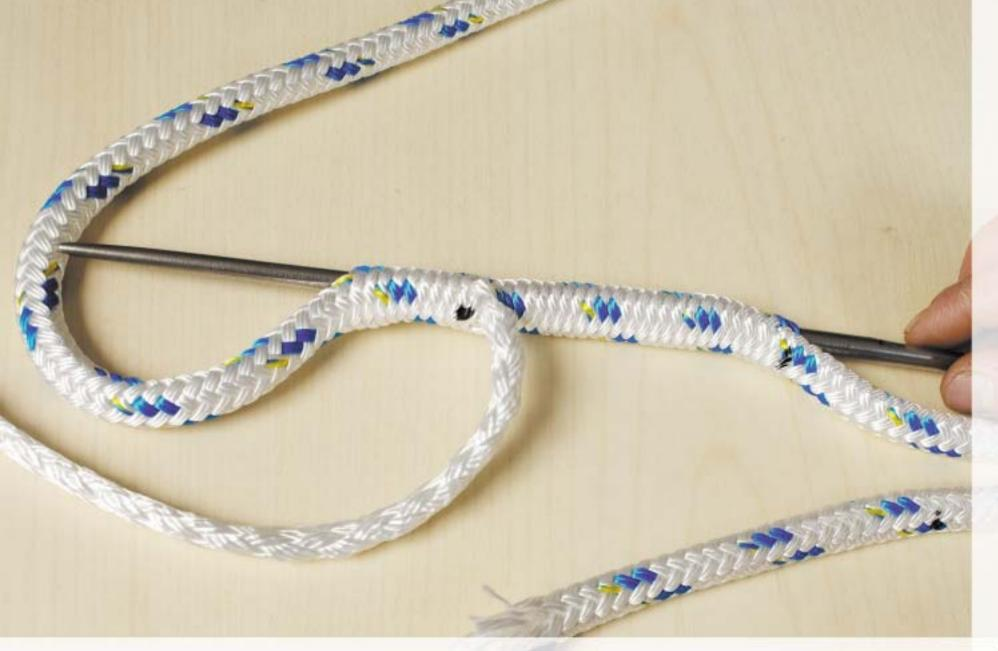
Feed the core into the fid and isert at the 15 cm mark and push it through towards the 30 cm mark where the core comes out. If possible make the exit 20 cm beyond the 30 cm.
