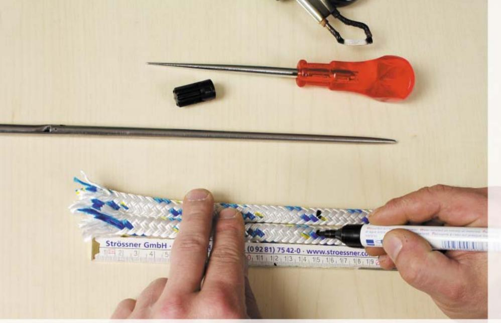
Mark both ends of the rope at a point 15 x 30 cm from each end of the rope to be spliced.
