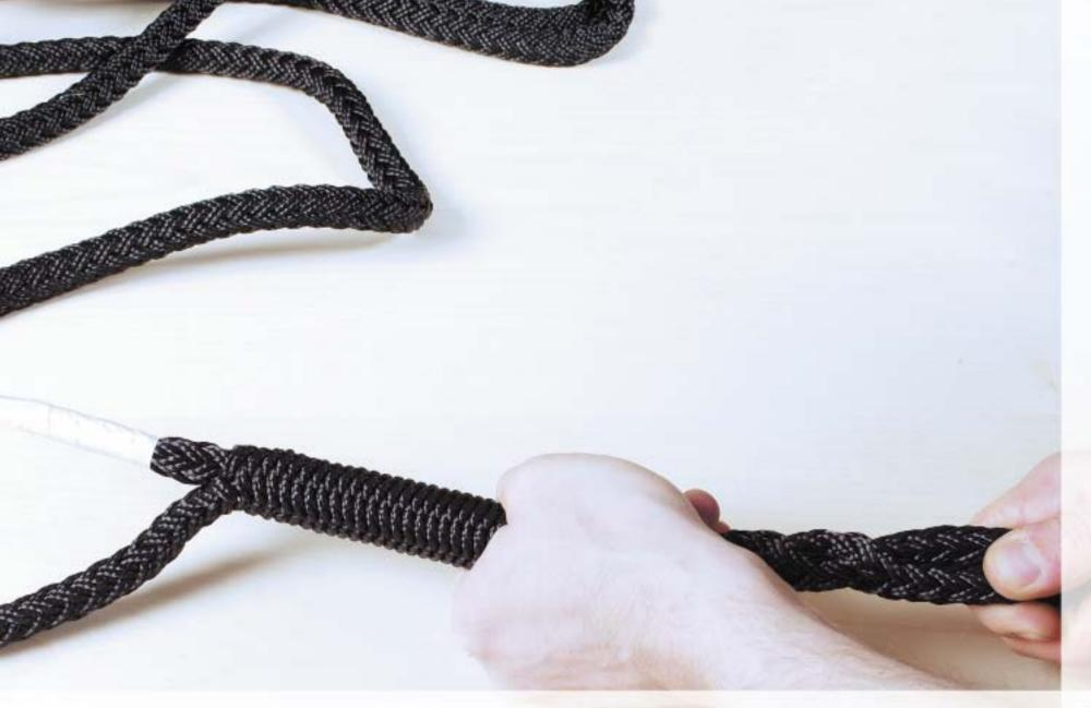
Remove the tape from the pointed tip and milk the cover so the end disappears.
