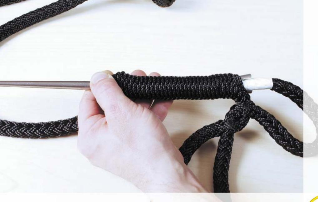
Pull the splicing tool all the way down. Its entire length and then extract it.
