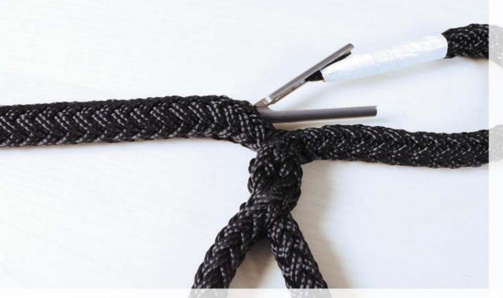
Now wedge the taped end into the splicing tool and push it down the core.
