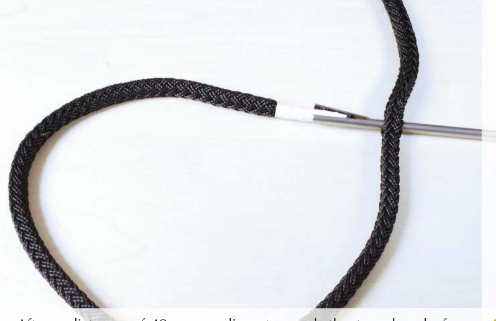
After a distance of 40 x rope diameter push the taped end of the rope through the fixed part of the rope and pull it tight using the splicing tool.
