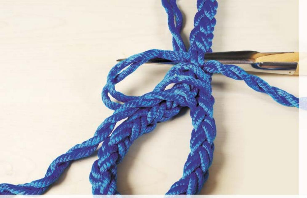
Using the fid insert the two strands from the left under the two strands.
