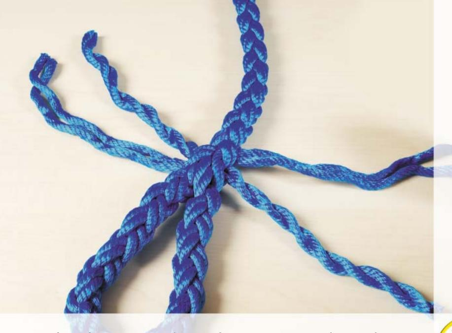
Make sure that the 4 pairs of strands are positioned exactly as per the picture.
