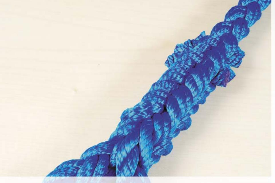
Photo showing the finished splice. The protudingends will disappear once the rope is used under tension.
