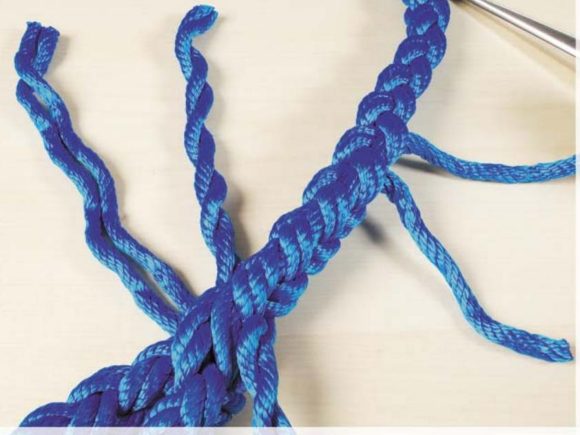
Make four further tucks down the rope with the first pair of strands. On the last tuck divide the pair into single strands so the splice becomes tapered.
