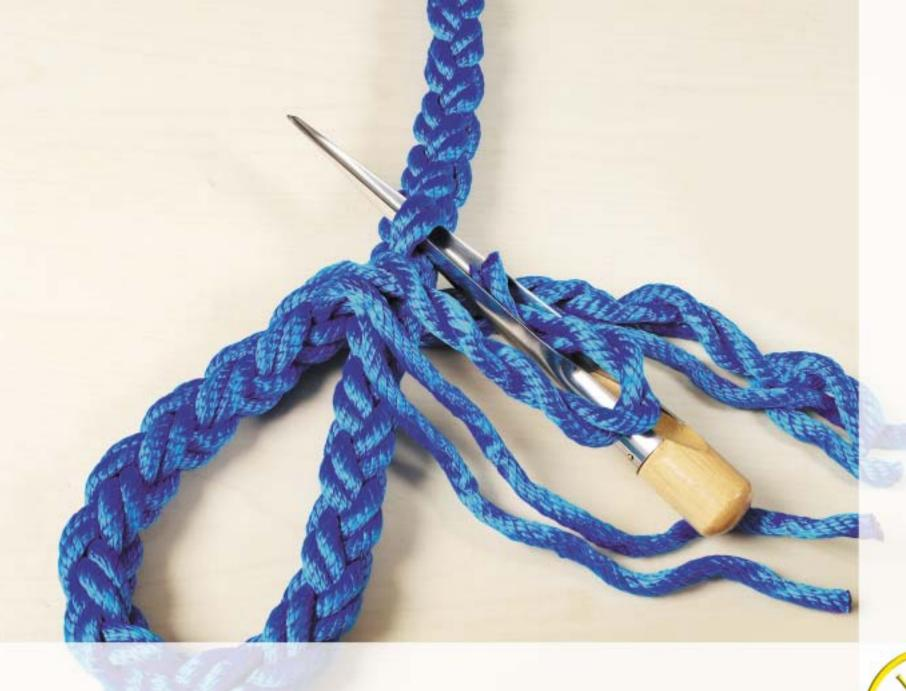
Insert the fid under two strands and feed the first pair through.
