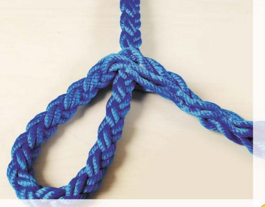
Measure the size of loop required. Then lay half the strand over and the other half under the rope.
